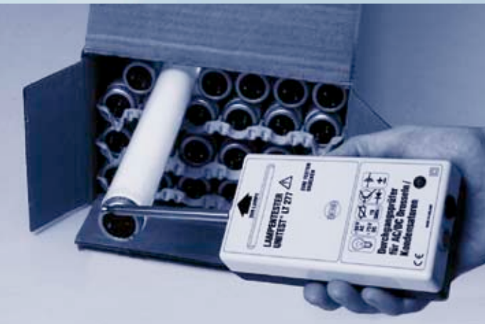
Quality management: test of single lamps
