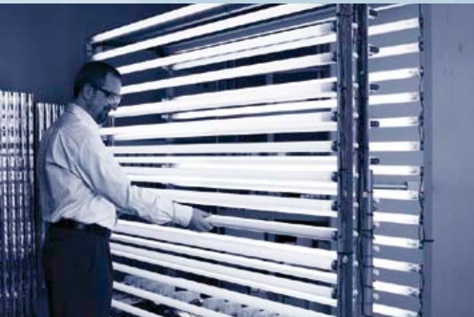
Quality management: lifetime tests in Stuttgart
